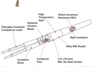
\* First 2 in. (51 mm) at lead end must be kept below 1000°F (538°C)
