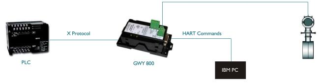
2. HART Transmitters as slaves on Modbus network using single GWY-800
