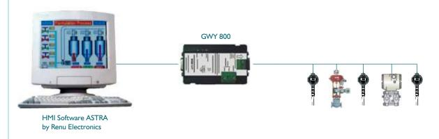
3. HART Transmitters as slaves on Modbus network using multiple GWY-800
